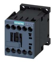
Power contactor, AC-3 7 A, 3 kW / 400 V 1 NC, 230 V AC, 50 / 60 Hz 3-pole, Size S00 screw terminal
