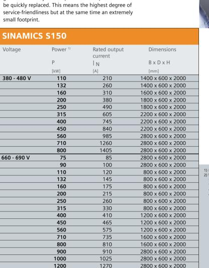
1) For 400 V or 690 V supply voltage 2) The cabinet height is increased by 250 mm for degree of protection IP21, by 400 mm for degrees of protection IP23, IP54 and by 405 mm for line supply options or motor connections from the top.
