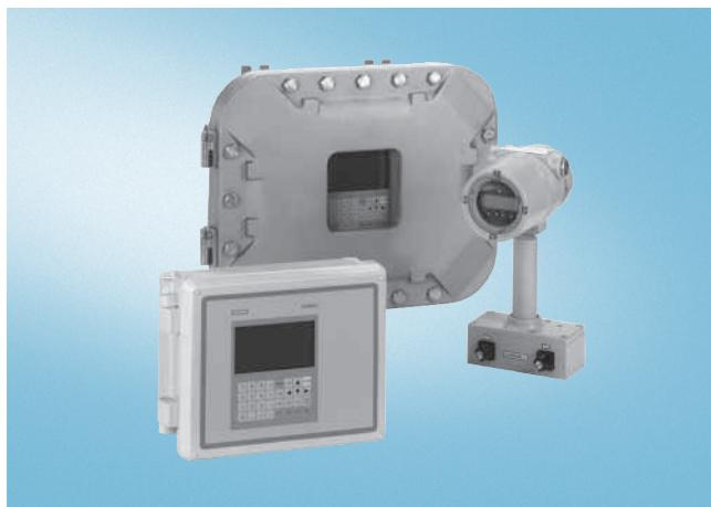
SITRANS FUS1010 is the most versatile clamp-on ultrasonic flowmeter available today. It can operate in either WideBeam Transit-Time or Reflexor (Doppler) mode, making it suitable for virtually any liquid, even those with high aeration or suspended solids.
