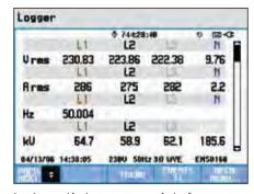
Logging provides instantaneous analysis of user selectable parameters.
