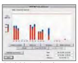
The included PQ Analyze software provides a detailed overview of several power quality parameters on one dashboard according to the EN50160 power quality standard.
